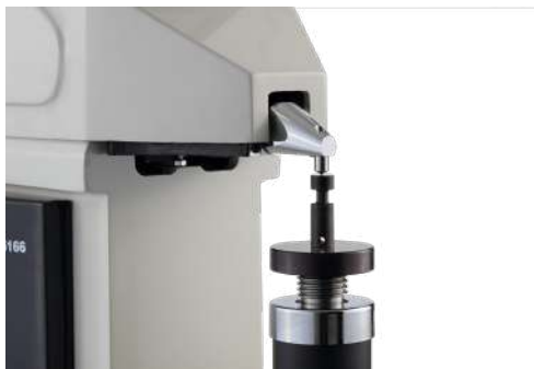
Ring/pipe inner wall hardness test
