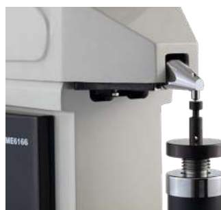
Surface hardness test of pin shaft
