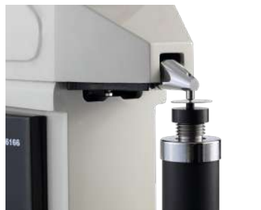
Use diamond specimen support to test HR30Tsm and HR15Tsm of thin tin plate
